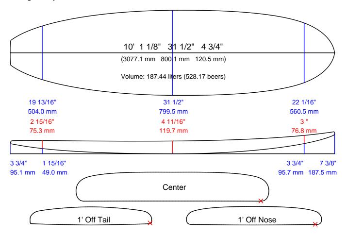
Measurements are center, one foot in and one foot back, over curve.
